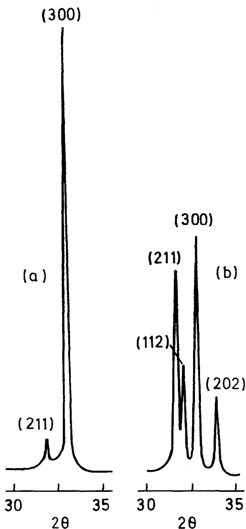
Fig. 2. XRD patterns of calcium hydroxyapatites obtained from \text{Ca}(\text{NO}_3)_2 0.05 M, pH = 11, R = 1 , 200°C and aging time 1 h. (a) Oriented aggregate films, (b) non-oriented.
